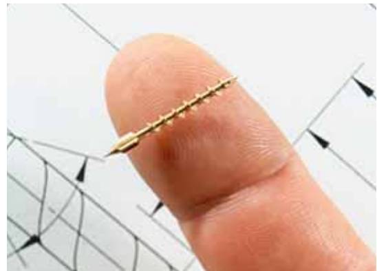
This approx. 1.5 cm long high-precision atomizer shaft made of brass for a textile machine was manufactured on a Tornos Deco 2000 shortly after a series of stainless steel parts using the same cutting oil (Ortho NF-X).
